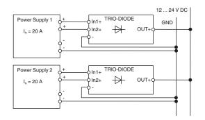
One redundancy module per power supply is required to decouple power supplies with nominal currents from 10 A to 20 A. Inputs "In1+" and "In2+" of the redundancy module must be connected to the power supply unit using two conductors. This is necessary because the maximum current carrying capacity of 15 A per input must not be exceeded. For connecting the redundancy module to the power supply unit, we recommend using two identical connecting cables (cable length/cable cross sections).
